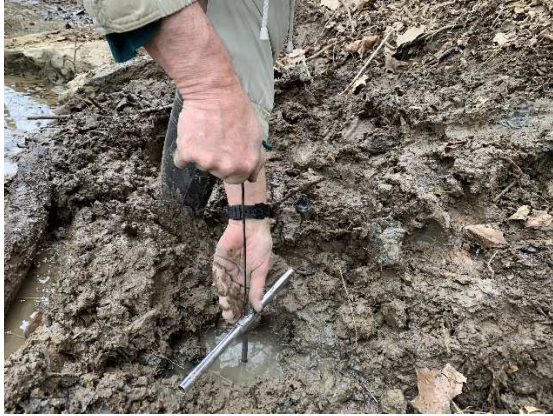
Figure 9 - Cores were extracted from several of the timbers using an increment borer. The cores were taken to the lab at Virginia Tech for species identification.
