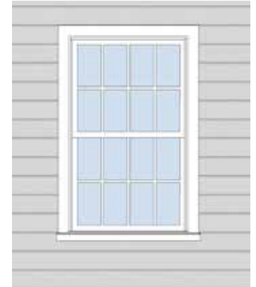
Eight-over-eight sash in 20th c. revival styles.
