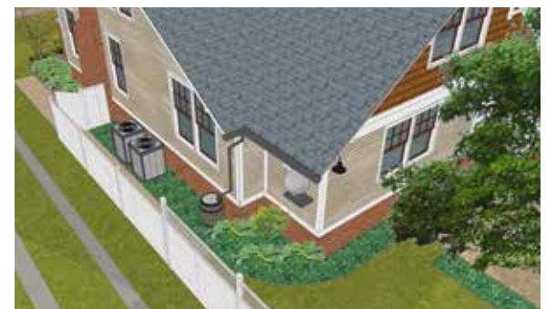
Typical side locations of HVAC equipment should be screened with landscaping &/or fences if possible.
