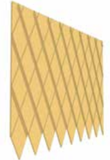
Diamond patterned shingles are found on several dwellings in the historic districts.
