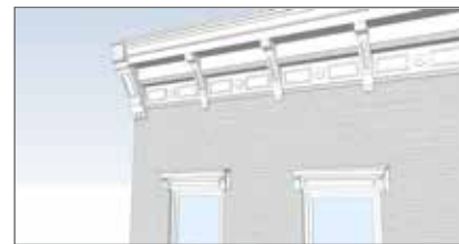
A typical Italianate commercial projecting cornice consists of curved brackets separating decorative panels.
