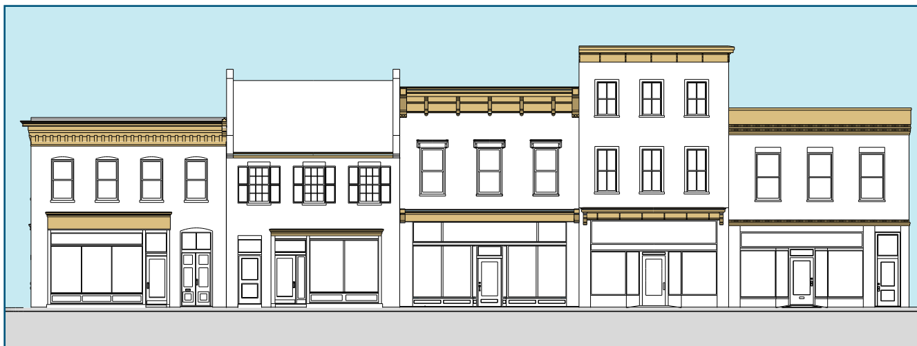
Most historic commercial buildings have cornices at the storefront level & at the roof line, as illustrated here.
