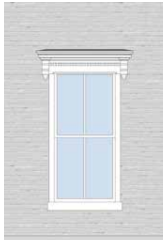
Two-over-two sash in a brick building with decorative cap.
