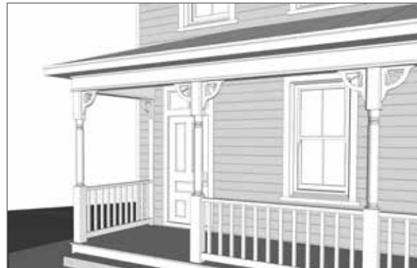
More decorative porches date from the mid-to-late 19th c. & may contain brackets, turned posts, & other sawn millwork details.
