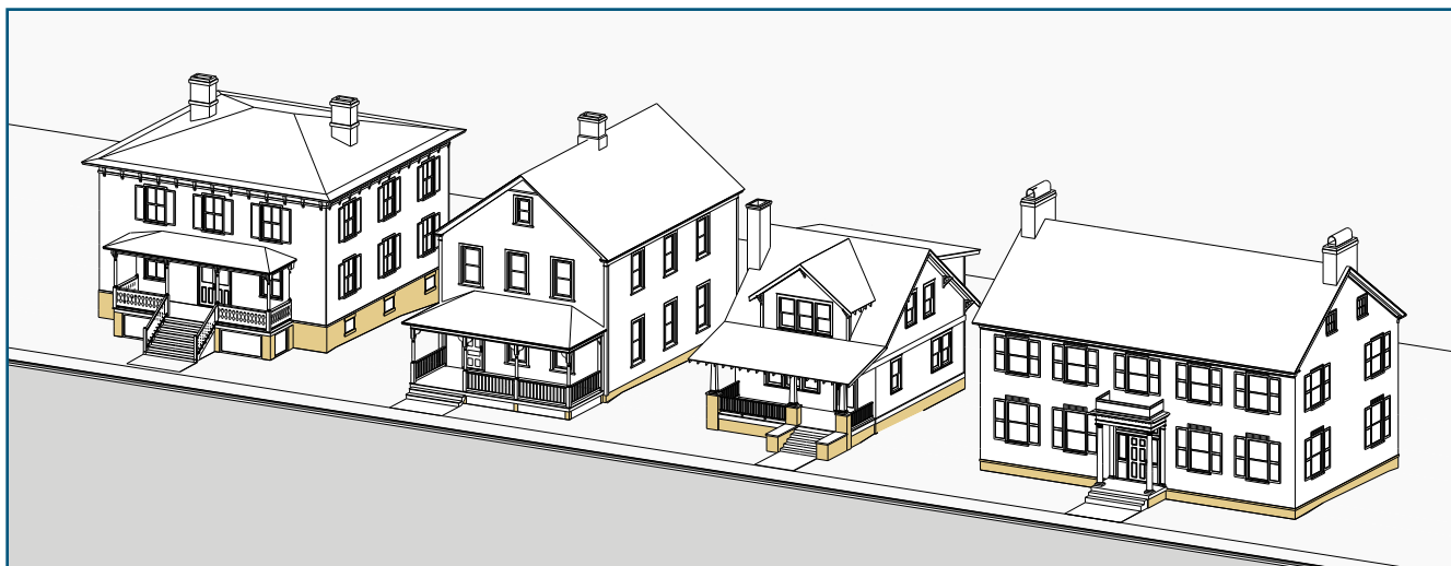
Most historic houses have the foundation articulated with a different material, or different treatment of the same material, that visually sets the building on a level base.
