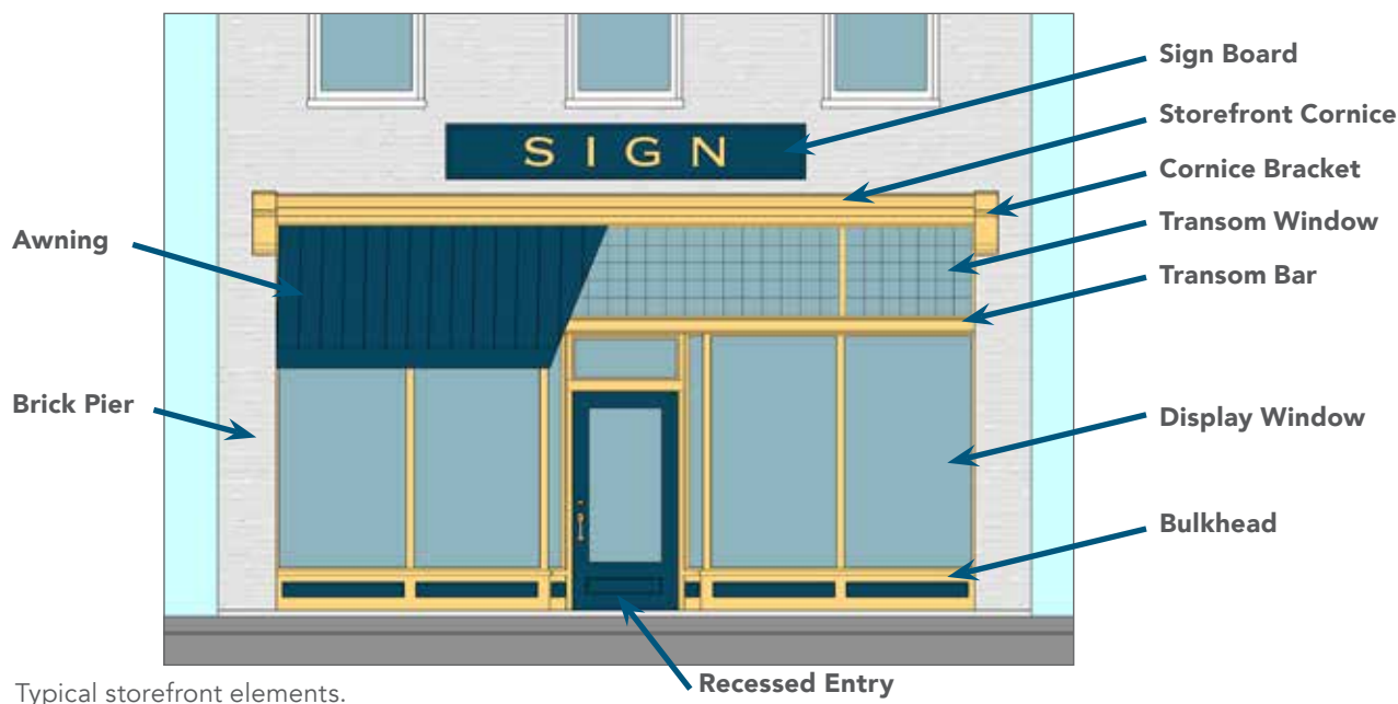
Typical storefront elements.
