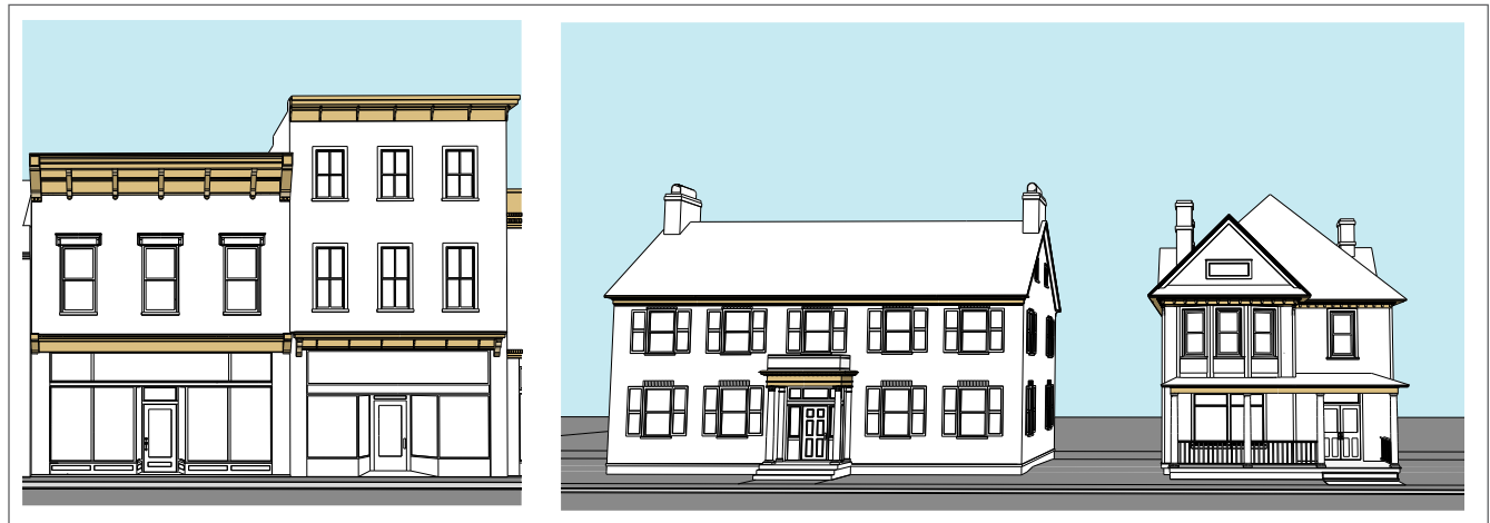
Cornices are major character defining features on both commercial & residential buildings in Lexington’s historic districts.
