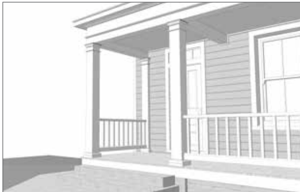
This simple full-width porch is often seen on a Folk Victorian, American Foursquare, or vernacular dwelling.
