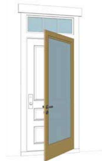
This storm door is a single pane of glass to allow the door underneath to be seen. It could also have divisions to match the historic door.
