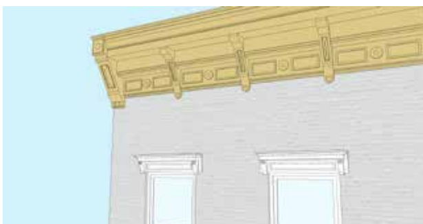
Commercial cornices may be simple or more detailed with brackets & decorative panels, as in this example.
