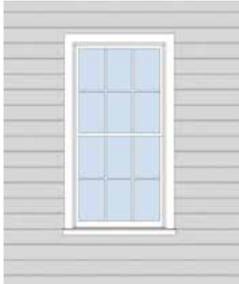
Six-over-six sash in earlier & in revival styles.
