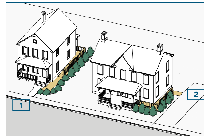
Depending on site conditions and topography, a ramp can be added at the front sidewalk to access a building's rear entrance (Example 1). Example 2 shows a ramp beginning at a driveway to provide access at the front porch. Landscaping in both examples is used to mitigate the appearance of the ramp on historic buildings.
