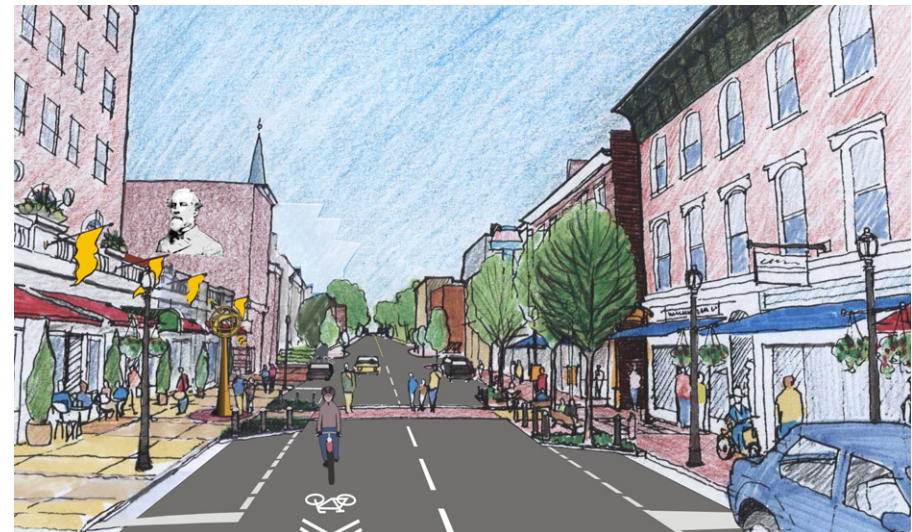
The mid-block crossing links with the pedestrian alley to McCrum's parking lot. This feature allows for pedestrians to safely cross the street while providing shade and creating areas to stop and linger. This sketch also shows sharrows along Main Street.
