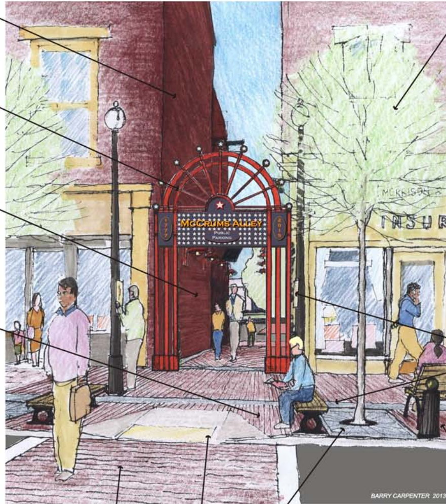
Pedestrian Crosswalk With Special Paving Handicapped Ramp Tree Grate
