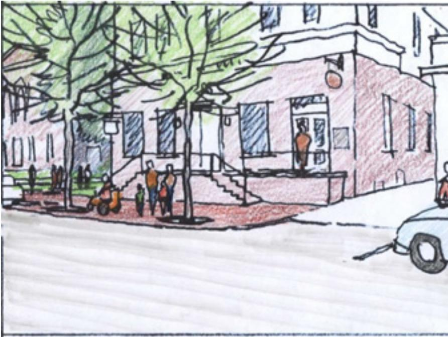
Consider cost reduction strategies such as: Allowing utilities to remain under sidewalk extensions, use of trench drains (channels covered with metal grating), and allowing fire hydrants to remain in place whenever reasonable; bulbouts keep area clear of illegally parked cars, improving access to hydrants.
